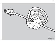
5 Attach the network cable to the 10BASE-T/100BASE-TX port on the machine.
